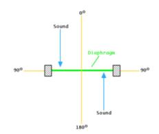
Sound that impinges from 0° or 180° has to travel an extra distance around the diaphragm to reach the rear side. This produces a pressure different between front and rear of the diaphragm that causes the diaphragm to experience a force. The algebraic sign differs for 0° and 180°.
