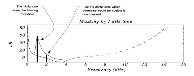
The reason for frequency masking arises from the functioning of our hearing. The inner ear performs some kind of spatial frequency analysis. Different parts of the basilar membrane are associated with different frequencies. As each tone sets into vibration a certain area of the basiliar membrane, a weaker tone with similar frequency may not be detected.
