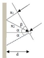
Reflected wave travels a distance  $(x_1+x_2)$  longer than the direct path.
