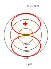
b) 1: Place an omnidirectional microphone coincident with a figure-of-eight and add the output signals
