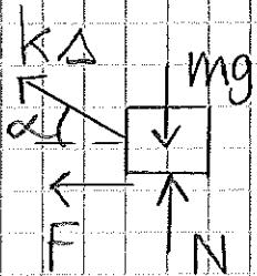
$$\begin{aligned} \uparrow: N - mg + k\Delta \sin \alpha &= 0 \quad (1) \\ \leftarrow: F + k\Delta \cos \alpha &= ma_n = mL\omega_0^2 \quad (2) \\ \Delta &= L / \cos \alpha - L \quad (3) \end{aligned}$$
