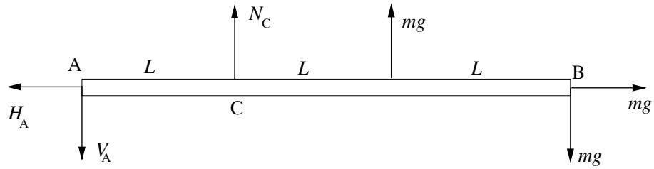
$$\begin{aligned} \leftarrow & H_A - mg = 0, \\ \downarrow & V_A - N_C - mg + mg = 0, \\ \curvearrowright & N_C L + mg \cdot 2L - mg \cdot 3L = 0. \end{aligned}$$
