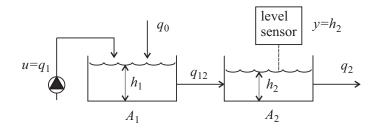
According to Bernoulli's law the flow between the two tanks is given by
