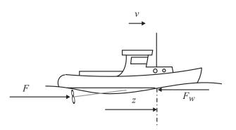
Let the boat position be z(t) [m], the boat speed be v(t) [m/s] and the propulsion force be F(t) [N]. We may assume all friction forces together be related to the speed according to
