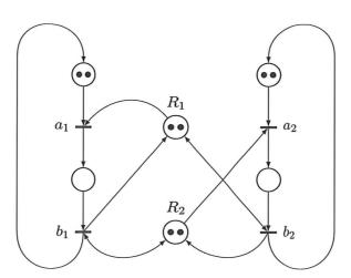
a) Generate the reachability graph of this Petri net (PN) and identify the blocking states when the initial marking vector is the marked state.
