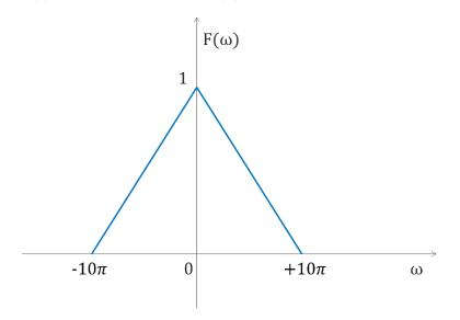
with  $\omega$  expressed in radians / second, plot the Fourier spectrum  $\overline{F}(\omega)$  of the signal  $\overline{f}(t)$  obtained by sampling the signal f(t) at a rate of  $\omega_s = 15\pi$  r/s. Motivate your answer.
