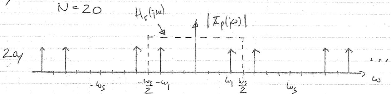
b)  $y(t) = x(t) = \sin(\omega_1 t)$        $\omega_1 < \frac{\omega_s}{2}$       No aliasing
