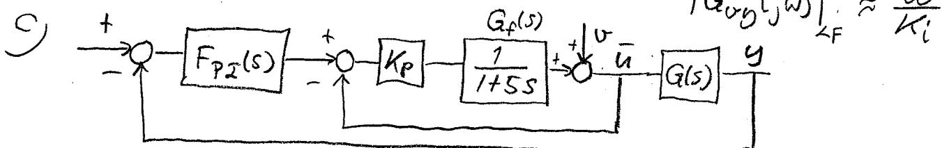
$$Y = G\bar{U} \quad \bar{U} = V + G_f K_p (-\bar{U} - F_{P2} G \bar{U}) \quad (1 + G_f K_p (1 + F_{P2} G)) \bar{U} = V$$
