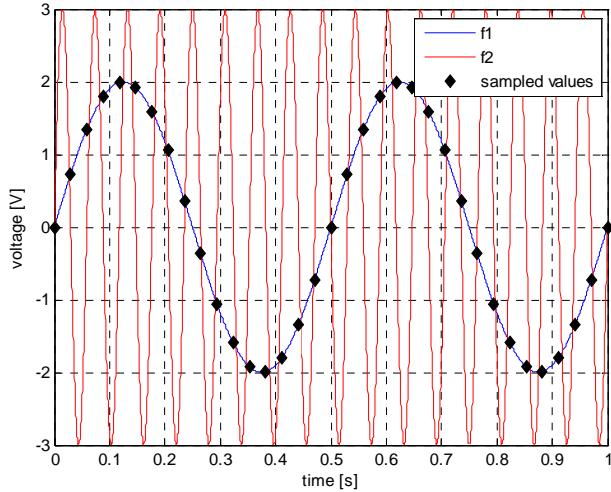
$$f_s > 2f_{max} \rightarrow f_{max} < \frac{f_s}{2} = 17 \text{ Hz} \text{ (in practice } f_{max} < \frac{f_s}{4})$$
