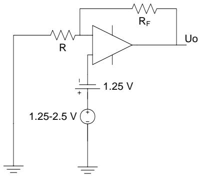
$$V_o = \left(1 + \frac{R_F}{R}\right) (V_i - 1.25) \text{ for } V_i = 2.5, V_o = 5 \rightarrow \frac{R_F}{R} = 3$$
