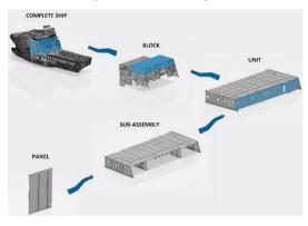
sub-assemblies, units, blocks and then the blocks are welded to a complete ship.
