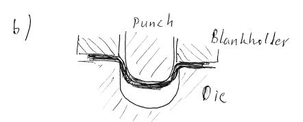
Blankholder force controls wrinkling but lets the material slide in to the die
