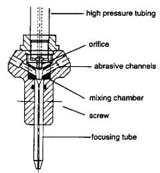
Process parameters: Water pressure, abrasive mass flow rate. Orifice and nozzle diameters
