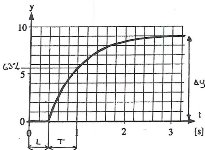
$$\begin{aligned} \text{Inignalsteg } \Delta u &= 0,5 \\ \text{Ur stegsvar } \Delta y &= 9 \end{aligned} \quad \left. \right\} \Rightarrow k = \frac{9}{0,5} = 18$$
