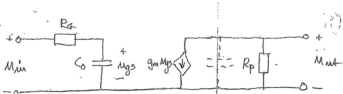
$$C_0 = C_{M1} + C_{gs} = 324 \mu F + 30 \mu F = 354 \mu F.$$
