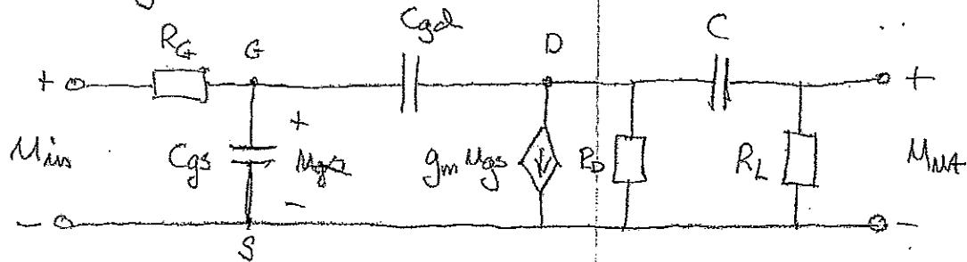
$$R_G = 800\Omega, R_D = 4k\Omega, R_L = 4k\Omega, C = 200\text{nF}$$
