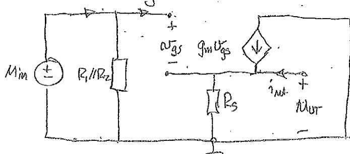
$$U_{in} = U_{gs} + g_m U_{gs} \cdot R_s, \quad M_{out} = g_m U_{gs} R_s \Rightarrow$$
