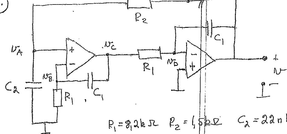
$$R_1 = 8,2 \text{ k}\Omega \quad R_2 = 1,5 \text{ k}\Omega \quad C_2 = 22 \text{ nF}$$
