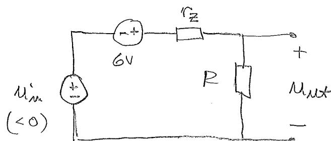
$$R = 20 \Omega \quad r_Z = 2 \Omega \quad M_{im} = 12 \cdot \sin \omega t \text{ V}$$
