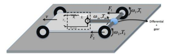
with mass m and velocity v. The vehicle velocity is regulated by varying the input voltage to the electric motor  $V_{in}$ .
