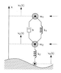
where  $m_1$  and  $m_2$  are the masses of the vehicle and the wheel, respectively,  $k_1$  and b = b(u) are the spring and friction constants, respectively, of the suspension, u is an exogenous signal and  $k_2$  is the spring constant of the wheel.
