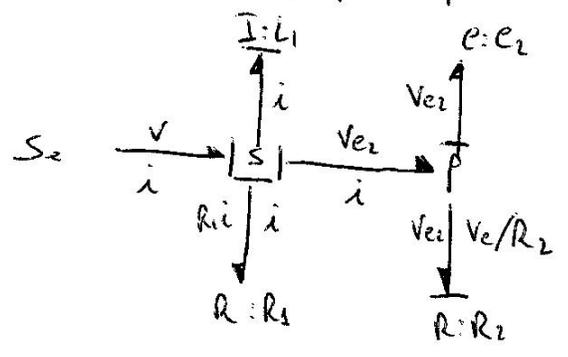
$v(t)$  should be selected as input signal, ~~source~~ otherwise a step change in the current signal would result in large voltage in the  $I$  element.
