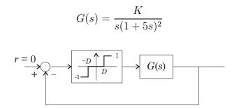
The deadzone parameter D is a design parameter for the thermostat. If it is too small the system will oscillate. Approximately how large does D have to be to avoid self-oscillation.
