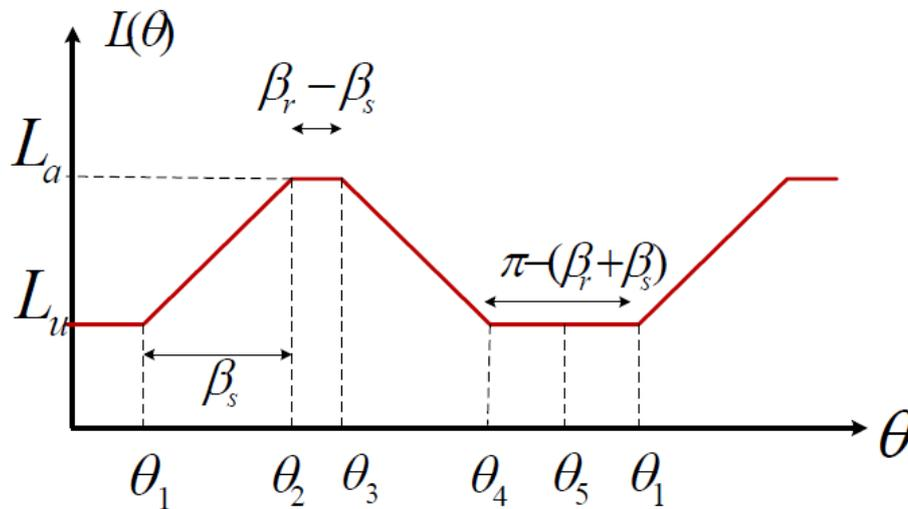
d) The torque is  $T_e = \frac{1}{2} i^2 \frac{dL}{d\theta}$ . For this motor the value is  $\frac{1}{2} 10^2 \frac{(600 - 100) \mu\text{H}}{\frac{\pi}{6}} = 0.4774 \text{ Nm}$ .
