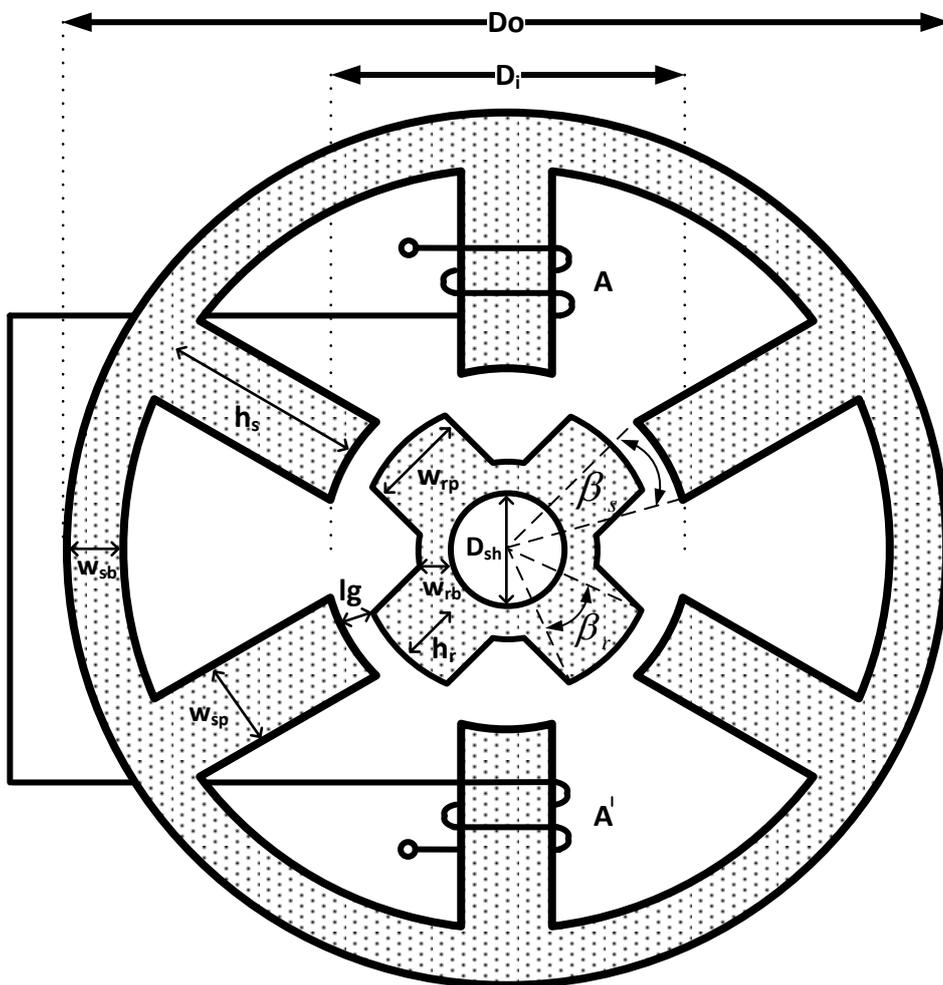
Figure 1: Cross section diagram of a SRM
