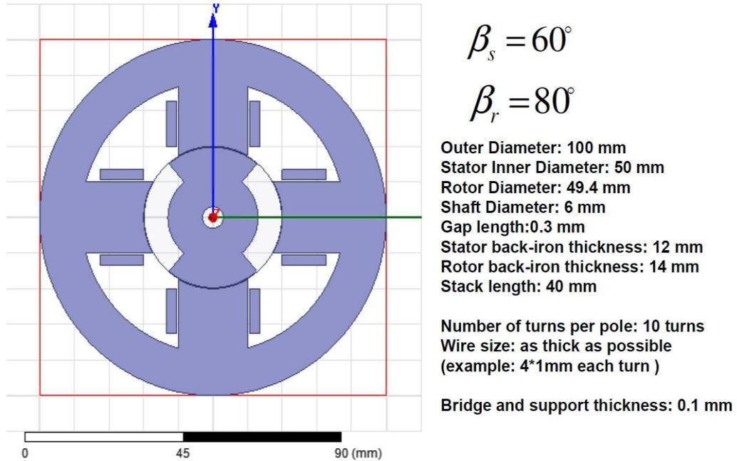
**Fig Q4-1: Geometrical information of a 4/2 SRM**
