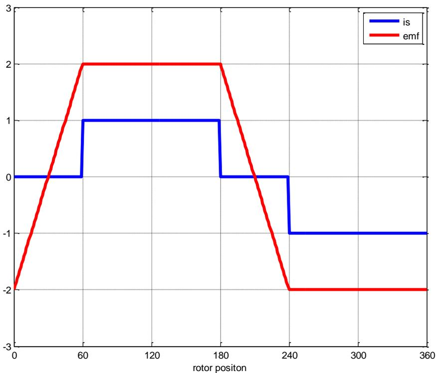
b) Since only two phases are active at every time instant (except for the time when two phases commutates), The equivalent circuit of the BLDC motor can be represented by two phases in series all the time.
