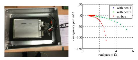
At this high frequency is the inductance that governs the behaviour. (Also parasitic capacitance as well as the skin effect impact on the resistance is evident)
