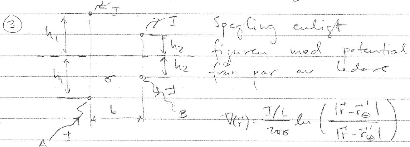
$$\nabla_A = \frac{I/L}{2\pi\epsilon_0} \ln \left( \frac{\sqrt{b^2 + (h_1 + h_2)^2}}{a}, \frac{\sqrt{b^2 + (h_1 - h_2)^2}}{2h_1} \right)$$
