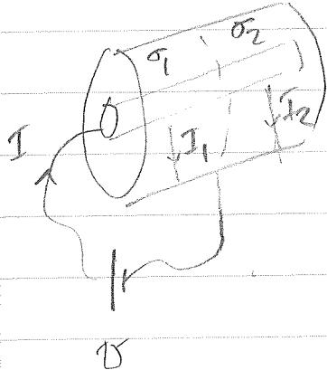
$$\begin{aligned} J &= J_1 + J_2 = \int_{S_1} \vec{J}_1 \cdot \vec{ds} + \int_{S_2} \vec{J}_2 \cdot \vec{ds} \\ &= 2\pi rh J_{r_1}(r) + 2\pi r(L-h) J_{r_2}(r) \end{aligned}$$
