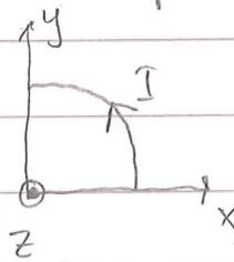
$$\vec{B}_{xy}(r=0) = \frac{\mu_0}{4\pi} \int_{xy} \frac{\vec{I}}{|\vec{r} - \vec{r}'|^2} \times \frac{\vec{r} - \vec{r}'}{|\vec{r} - \vec{r}'|} d\ell$$
