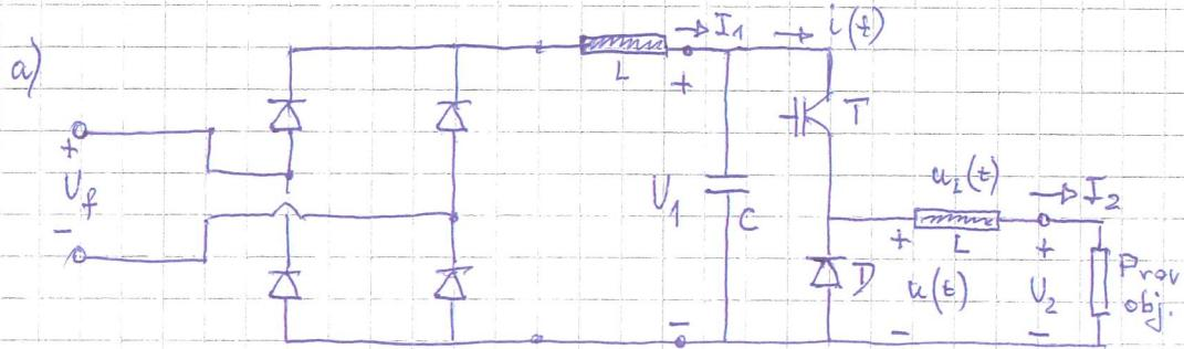
$$U_f = 230 \text{ V} ; U_2 = 120 \text{ V} ; I_2 = 6 \text{ A} ; f_{sw} = 100 \text{ kHz}$$
