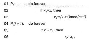
Figure 3 Dijkstra algorithm for token circulation
