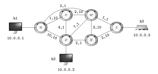
In the above network, each link connecting 2 routers is labelled  $\ell$ , *B* where  $\ell$  is a latency measure (in ms) and *B* is the bandwidth capacity of the link (in Gbps).
