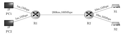
Above each link of the network is mentioned the values "D,B" where D is the length of the link and B is the bandwidth of the link. In this exercise, we will assume that:
