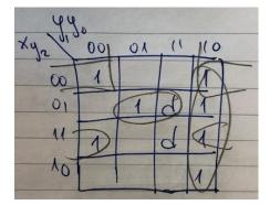
Z= y1 y0' + x' y2'y0' + x' y2 y0 + x y2 y0'
