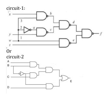
b) Draw a hazard-free equivalent of the circuit.
