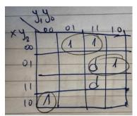
Y1= x y2' y1' y0' + x' y2' y0 + x' y2 y1
