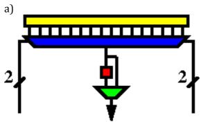
The yellow box is 16 bits of memory (or flip-flops), which together with the multiplexer implement a 4-input lookup table. The 4 bits inputs go to the select of the multiplexer. The output of the LUT goes to a flip-flip, and 2-to-1 multiplexer selects either the registered output or the one directly coming from the LUT.
