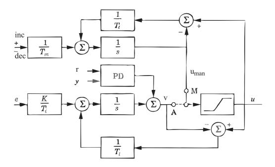
Write pseudo-code for implementing the PID-controller above. The derivation should act on the measured signal y only. Motivate any assumptions.
