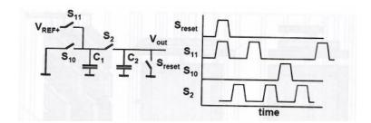
Bits  $(b_i)$  are processed in sequence, from the least to the most significant bit, and activate the switches  $S_{11}$  and  $S_{10}$  for values 1 and 0, respectively. After each step, the output voltage is given by:
