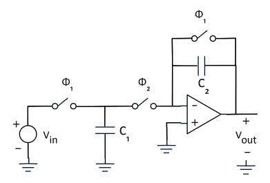
During  $\Phi_1$ , the input voltage  $V_{in}$  is sampled onto capacitor  $C_1$ , and the feedback capacitor  $C_2$  is reset. During  $\Phi_2$ , the input is disconnected and the charge on  $C_1$  is moved to  $C_2$ , such that the output voltage is  $V_{out} = -(C_1/C_2)V_{in}$ . The desired gain magnitude of the amplifier is 2. You may assume that the capacitors are perfectly matched.
