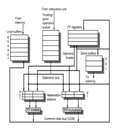
The above diagram shows a pipeline with Tomasulo's algorithm. Consider the following code:
