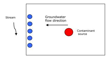
You have taken 5 samples of the groundwater contaminant concentration near the stream, represented by the five filled circles on the map. You got the following results: 9.33, 12.55, 45.21, 13.63 and 3.36 g/m<sup>3</sup>. You expect the hydrogeological conditions to be rather uniform over the area and at steady-state, i.e. concentrations are not expected to change over time. The flow in the small stream,  $Q_s = 0.03 \text{ m}^3/\text{s}$ .
